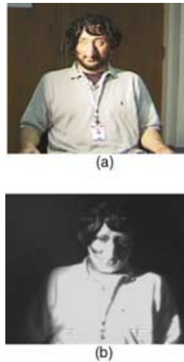
Figure 13. Appearance of a Caucasian individual wearing a total disguise in: (a) the visible spectrum and (b) the sub-band 1.3-1.7 \mu\text{m} of the upper near-infrared.
