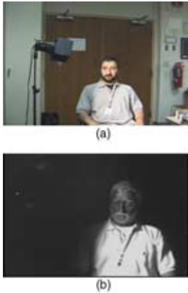
Figure 12. Appearance of an undisguised Caucasian individual in: (a) the visible spectrum and (b) the sub-band 1.3 – 1.7 \mu\text{m} of the upper near-infrared.
