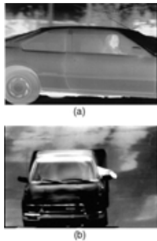
Figure 3. Snapshots of vehicles moving at low speeds (up to 15 mph) (a) Side view of a vehicle in the mid-infrared. (b) Frontal view of a vehicle in the mid-infrared.
